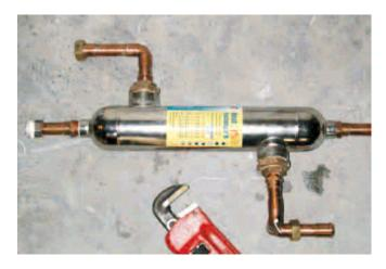
The liberal use of threaded unions allows for easy removal of components for repair or replacement.
