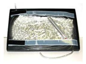
2. Place the clear rigid acrylic sheet on top of the assembled case. Tape the acrylic sheet to the case to make an enclosed space containing the aluminum foil, coiled tubing, and thermometer. This completes the assembly of the solar water heater panel.
