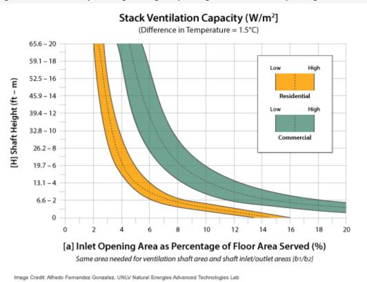
For example, a commercial building with a "Low" Building Classification, and an estimated ventilation stack height of 20 ft (6.1 m), the total area of the inlet opening would equal 6.8% of the total naturally ventilated floor area:
