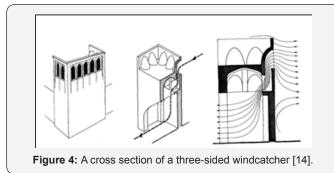
Figure 4 illustrates the three-sided wind catcher which often has larger windward side with more openings to capture as much predominant wind as possible. When air flow enters through the wind catcher, air velocity increases owing to curved form of openings.
