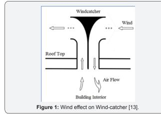
One of the conventional systems for providing natural ventilation inside the buildings without utilization of conventional energy is windcatcher. Over three thousand years, people in Middle East used the windcatchers for many buildings. They are known by various names like Badgir, Malghaf, etc. in different areas of this district.
