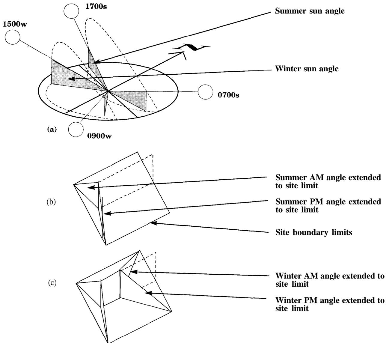
**Figure 2-4: Establishing Solar Envelope Boundaries**
