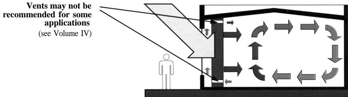
**Figure 1-8: Indirect Gain (IND) Schematic**
