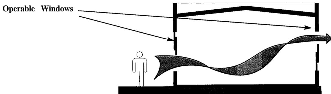
Figure 1-14: Natural Ventilation (NVN) Schematic
