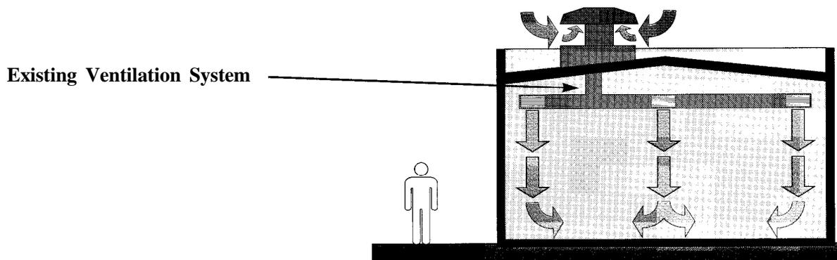
Figure 1-15: Night Mechanical Ventilation (NMV) Schematic
