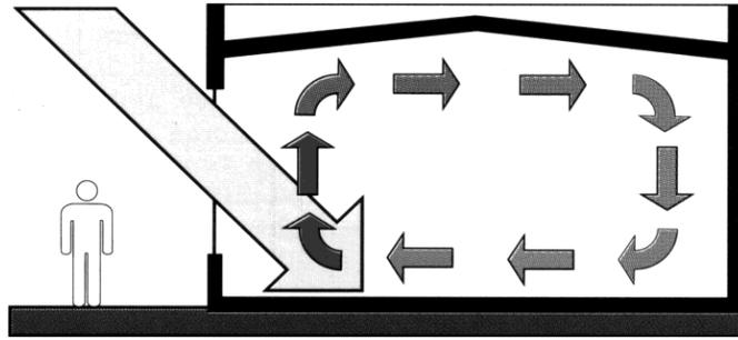
Figure 1-4: Direct Gain (DG) Schematic
