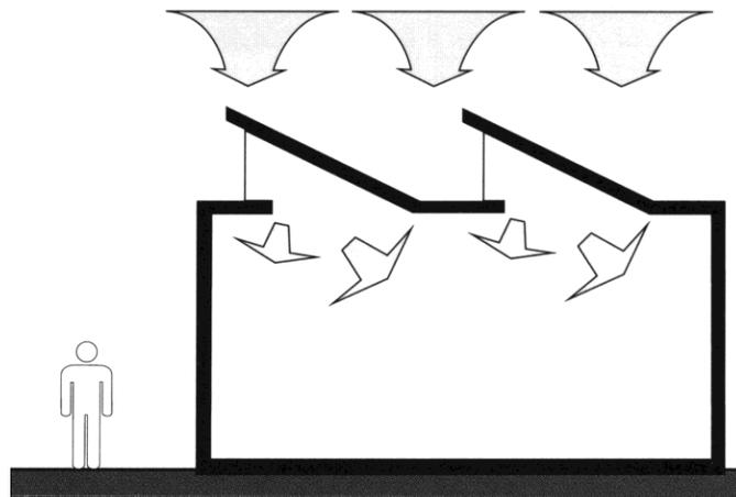
**Figure 1-21: Sawtooth Aperture (SAW) Schematic**
