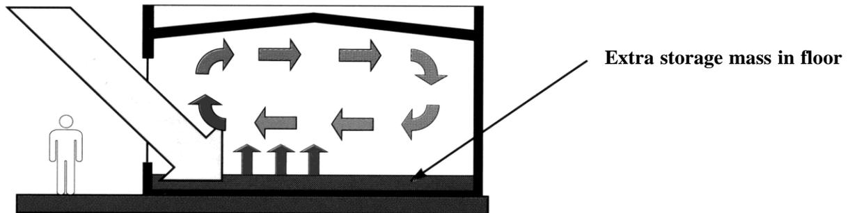
**Figure 1-6: Direct Gain plus Storage (D+S) Schematic**
