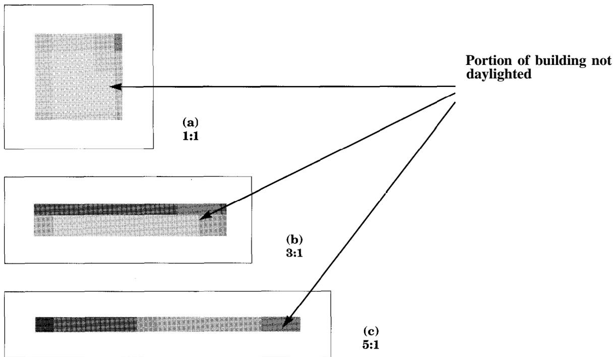
**Figure 2-11: Changes in Building Shape (Aspect Ratio)**
