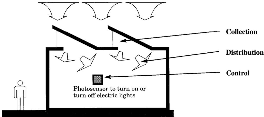
**Figure 1-3: Components of a Daylighting System**
