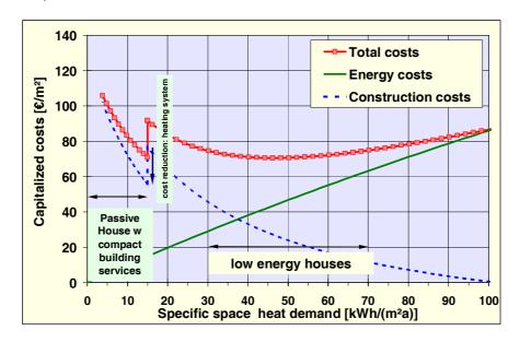
The primary function of the ventilation system is to maintain excellent indoor air quality. If the maximum load is lower than 10 W/m², the ventilation system can distribute all heat needed throughout the building as well. The definition of a Passive House is therefore that the peak heating load should be projected to a lower level than 10 W/m². In warmer climates, this value may be easy to achieve, however in colder climates, careful planning is required.
