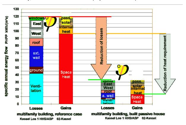
Examining the heating load is just one example. In other regions, other energy services, like cooling or dehumidification, could be of greater importance than heating. Again, the method for investigating a Passive House solution will be the following:
