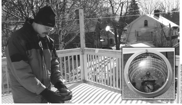
A site assessor uses a Solar Pathfinder to determine the effectiveness of solar energy at this home before the homeowner invests in a solar electric or solar hot water system. The inset photo to the right shows the Solar Pathfinder under ideal conditions.
