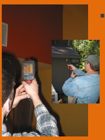
Shows major air leaks throughout house, especially where there's poor insulation
