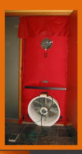
Helps find air leaks at windows, doors, can lights, floors, vents, etc.
