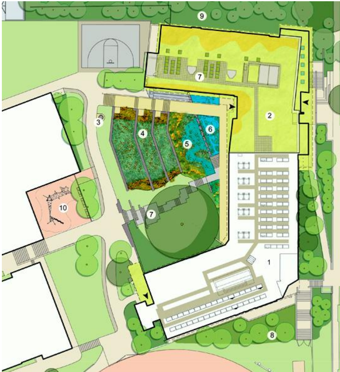
(Site plan: 1. Existing Middle School; 2. Middle School addition with green roof; 3. Trickle filter with interpretive display; 4. Wetlands for wastewater treatment; 5. Rain garden; 6. Pond; 7. Outdoor classroom; 8. Butterfly meadow; 9. Woodland screen at neighborhood edge; 10. Playground. Image by Andropogon Associates.)
