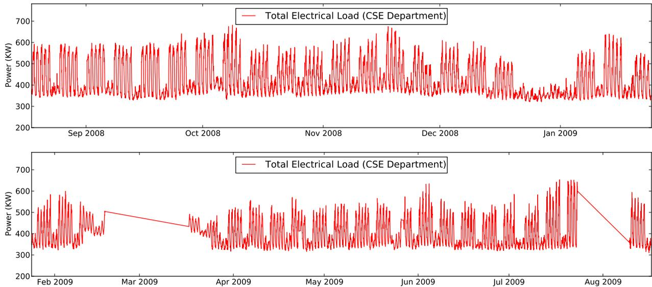
**Figure 3. CSE Mixed-use Building: Total electrical load for a year (August 18th, 2008 through August 16th, 2009). While the daily load varies by as much as 250KW, it never goes below 325KW. This is the base load of the CSE building. Due to data collection issues some data around March 2009 and August 2009 is unavailable.**
