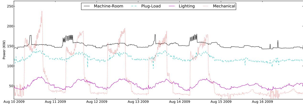
**Figure 5. Detailed breakdown of the energy consumption of the CSE mixed-use building. The data presented is for a week in August.**
