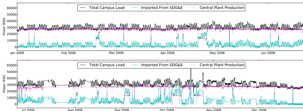
**Figure 1. UC San Diego Demand Response: Tracking the real time demand, total energy imported from SDGE, and the total energy production by the Central Utilities Plant in 2008.**
