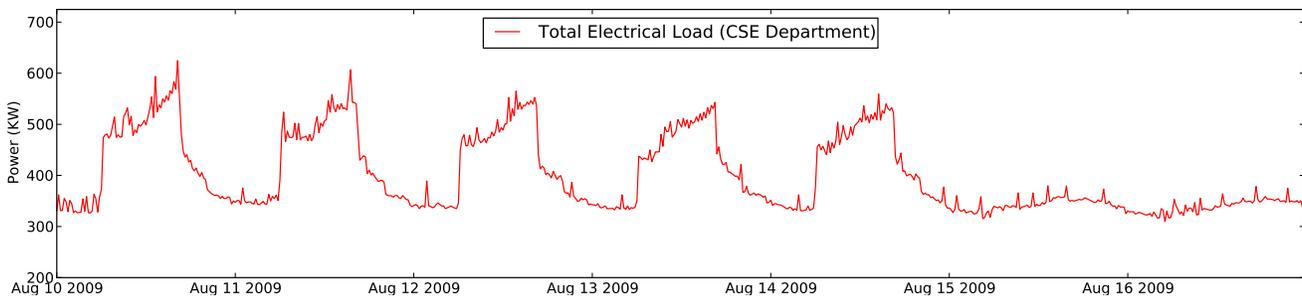
**Figure 4. Variation of the electrical load in the CSE building at UCSD during a week in August.**
