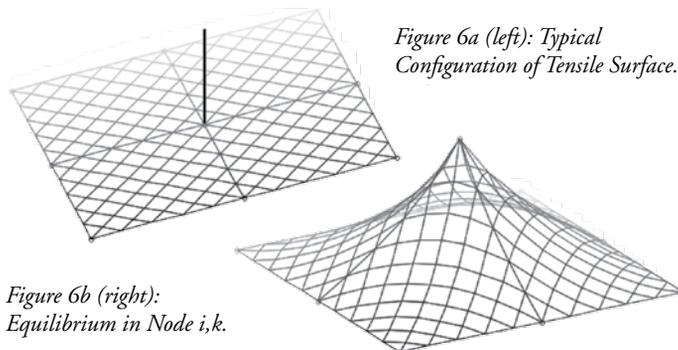
Figure 6a (left): Typical Configuration of Tensile Surface.
