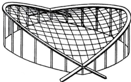
Figure 5: Cable Net of Raleigh Arena.
