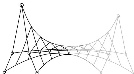
Figure 4: Stabilized Suspension.
