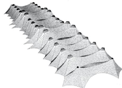
Figure 7: Geodesic Shape of the Denver Structure.
