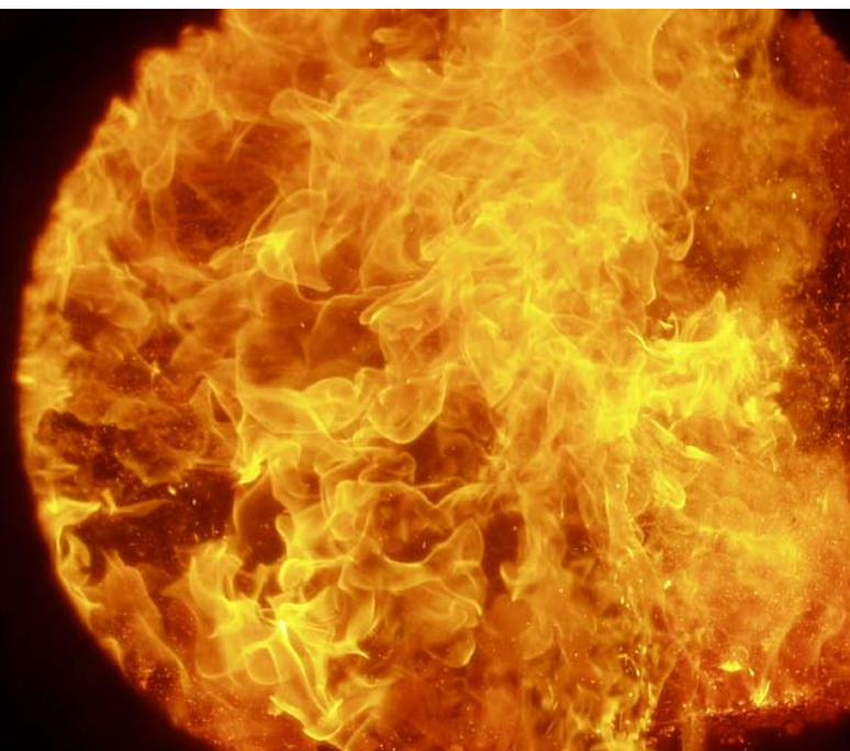
Forest chip during burning in grate furnace. Photo: SWECO Grøner AS.
