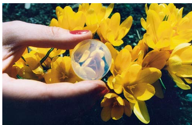
Monolithic aerogel produced at NTNU in Trondheim. Monolithic aerogels may be used in windows with high insulation and visibility performance.
