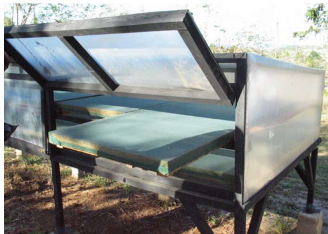
Solar dryer for fruits and spices in Tanzania. Photo: Jonas Sandgren.
