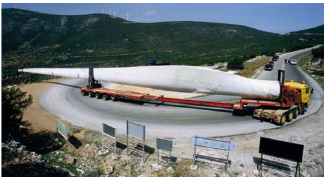
Transport of turbine elements to remote wind farms represents a considerable challenge. Often new roads and quay structures must be established. Photo: Vestas.
