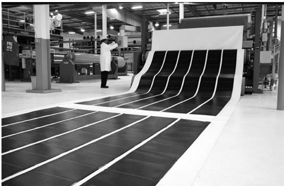
**Figure 3.26** A Manufacturing process for film technology. *Photo courtesy of Integrated Solar Technologies.*
