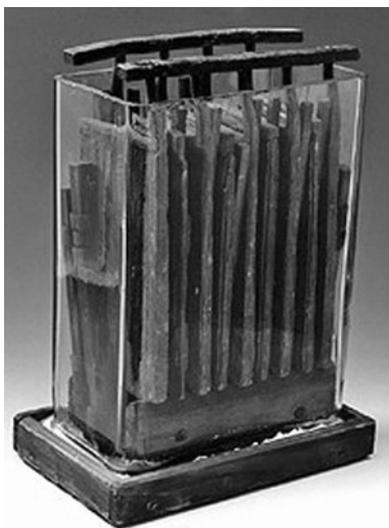
**Figure 3.40** Alessandro Volta's pile.
