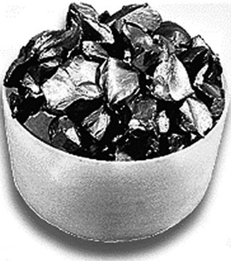
**Figure 3.15** Silicon crystals.
