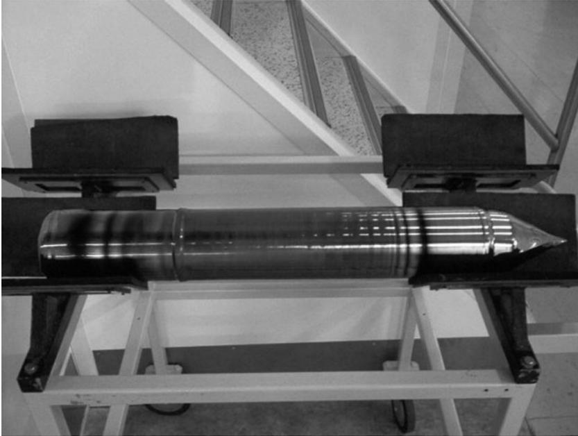
**Figure 3.17** A formed silicon ingot cylinder ready for inspection.
