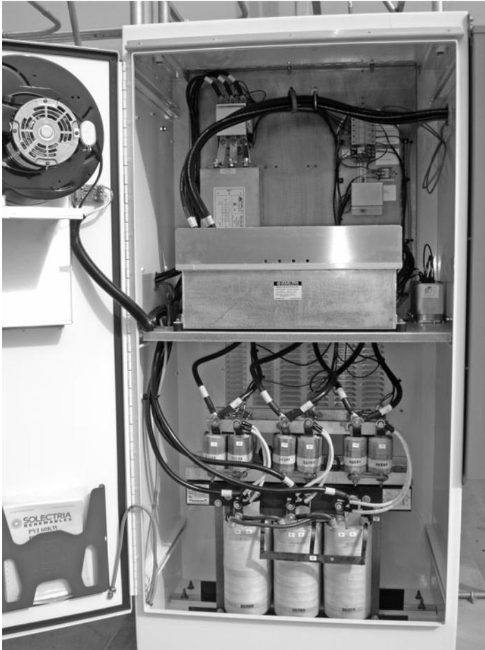
**Figure 3.13** Internal view of inverter electronics. *Photo courtesy of Solectria Renewables.*
