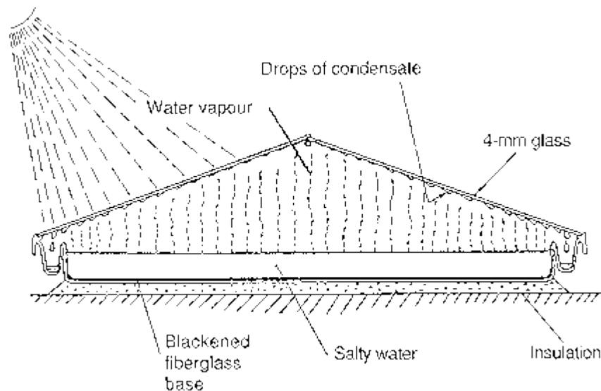
*Fig. 1. The Mexican still is simple, reliable, and efficient.*
